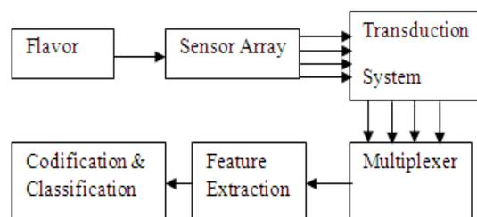
**Figure 1** Block representation of Electronic Tongue.
