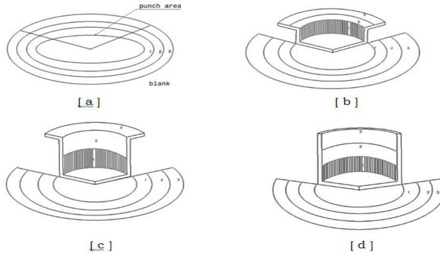
**Fig.1** Progression of metal flow in drawing a cup from a flat blanks
