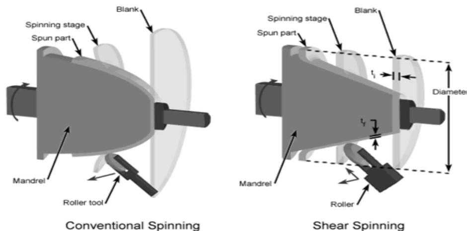
**Fig.3** Conventional Spinning and Shear Spinning process
