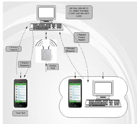
**Figure 1** Main component of a cloud framework
