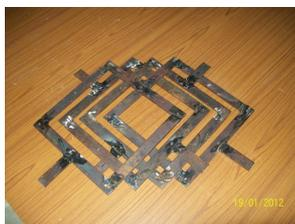
**Fig.5** Die to make FRP lay-up
