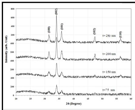
**Fig (1).** XRD for ZnO thin films deposited on glass substrates at different thicknesses.
