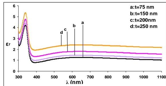
Fig.(6) Variation of  $\epsilon_r$  as a function of wavelength for ZnO films at different thickness
