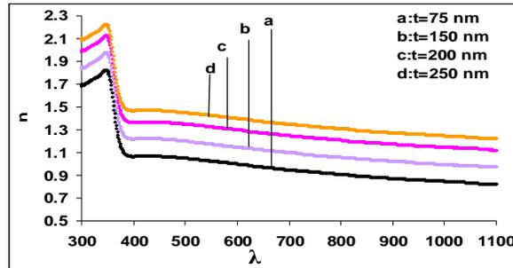
Fig(5) .Variation of n versus wavelength for ZnO films at different thickness.
