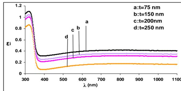
Fig. (7) Variation of  $\epsilon_i$  as a function of wavelength for ZnO films at different thickness.
