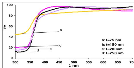
**Fig.(2)** Transmittance versus wavelength for ZnO films at different thicknesses.
