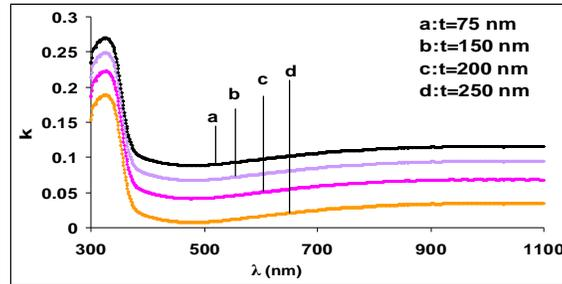
Fig(4) Variation of k versus wavelength for ZnO films at different thickness.
