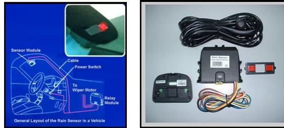
**Figure 2** Rain Sensor Wiper Systems [2]
