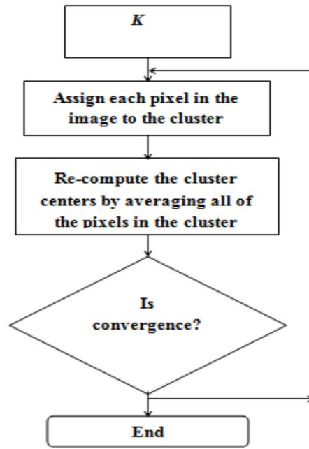
**Figure 1**Flow chart showing computation of clustering method.
