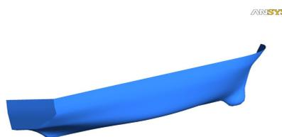
**Fig. 1** Geometry of free surface body after healing.
