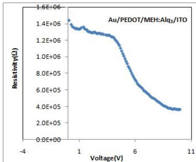
**Fig. 5.** Junction resistance vs. voltage graph of ITO/PEDOT:PSS/MEH:PPV/Alq3/Lif/Au Schottky diode
