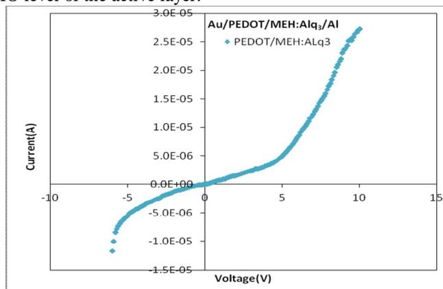
**Fig. 3** Current-voltage (I-V) characteristics of ITO/PEDOT: PSS/MEH:PPV/Alq3/Lif/Au Schottky barrier diode
