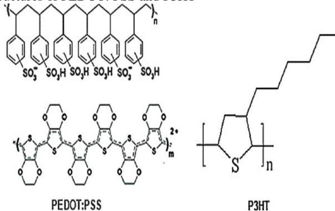
**Fig-1** Molecular structures of PEDOT:PSS and P3HT
