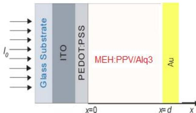
**Fig. 2.** Schematic layout of the ITO/PEDOT: PSS/MEH-PPV/Al photo detector on glass substrate
