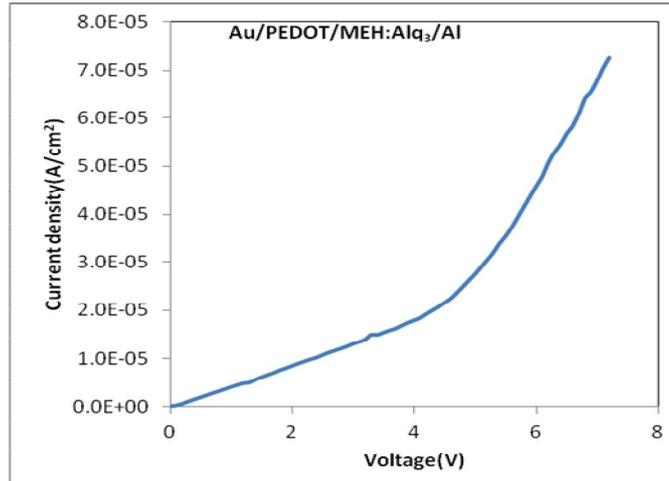
**Fig. 6.** Current density versus voltage for ITO/PEDOT: PSS/MEH: PPV/Alq3/Lif/Au Schottky diode.
