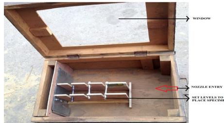
**Figure 5:** Shot Peening Environment for varying Nozzle tip distance (NTD)
