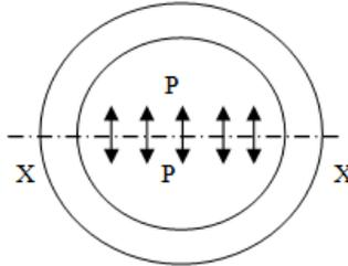
**Figure 1:** Hoop's stress on the vessel
