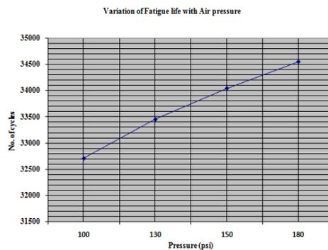
**Figure 11:** Variation of fatigue life with pressure
