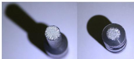
**Figure 12:** Fatigue failure of the specimen
