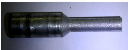
**Figure 9:** Surface of specimen after shot peening
