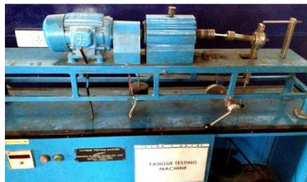
**Figure 7:** Specimen mounted in a rotary bending fatigue testing machine
