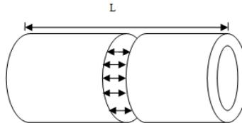
**Figure 2:** Longitudinal stress on the vessel
