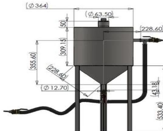
**Figure 3:** CAD model of portable shot peening machine
