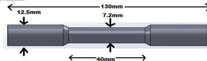
**Figure 6:** Dimensions of standard specimen (CAD Model)
