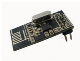
**Fig. 6** 2.4 Ghz RF Transceiver
