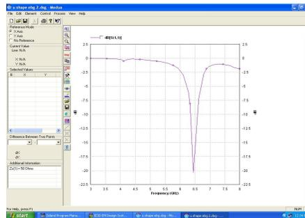
**Figure 5** Return loss ( $S_{11}$ ) of antenna with U slot EBG structure
