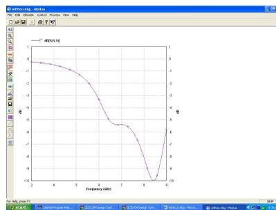
**Figure 2** Return loss ( $S_{11}$ ) of antenna without EBG structure
