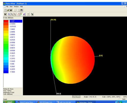
Figure 9 Radiation pattern of antenna with cross slot EBG structure
