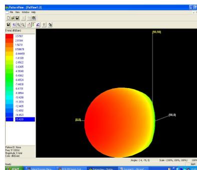
**Figure 3** Radiation pattern of antenna without EBG structure
