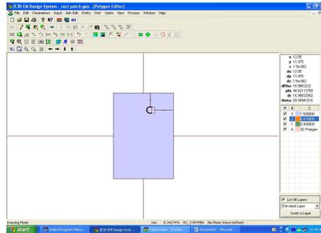
**Figure 1** Simple Patch Antenna with feed
