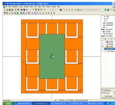
**Figure 4** Patch Antenna with U-shaped EBG slots
