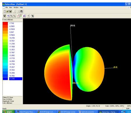
**Figure 6** Radiation pattern of antenna with U slot EBG structure
