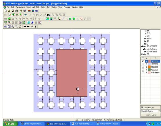
Figure 7 Patch Antenna using cross shaped EBG slots
