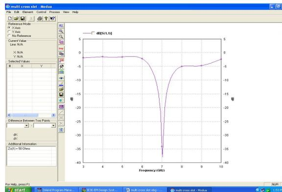
Figure 8 Return losses ( $S_{11}$ ) of antenna with cross slot EBG structure
