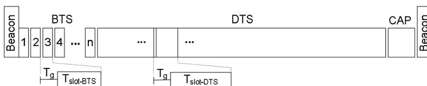
**Figure 6:** Proposed superframe structure including Beacon, Basic Time Slot field (BTS), Dedicated Time Slot field (DTS) and optional Contention Access Period (CAP) period
