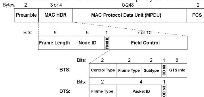
**Figure 7:** Proposed Packet Format for BTS and DTS fields
