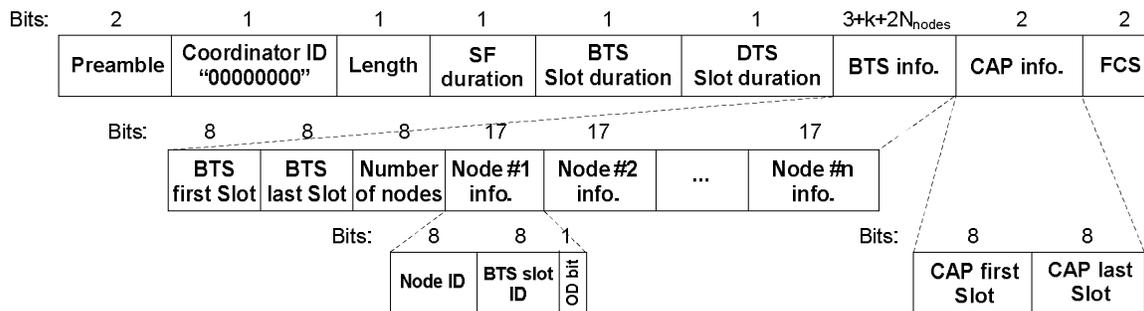
Figure 8: Proposed Beacon packet format
