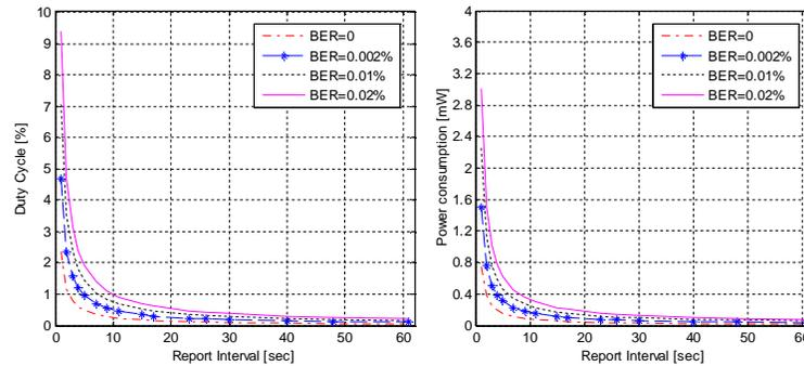
**Figure 9:** Duty Cycle and Power Consumption as a function of reporting interval, for various BERs
