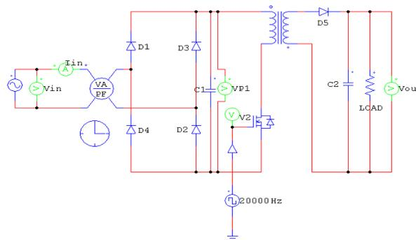
**Figure 5** SMPS using Fly-back topology
