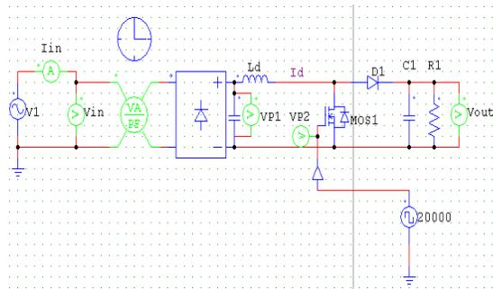
Figure 8 SMPS using boost topology
