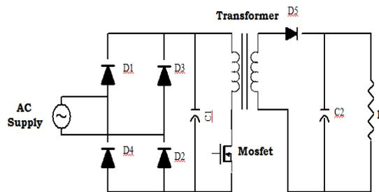
**Figure 2** SMPS using Fly-back topology
