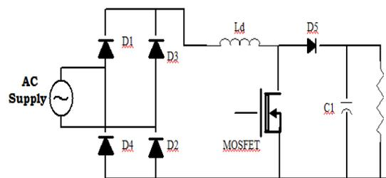
**Figure 3** SMPS using boost topology
