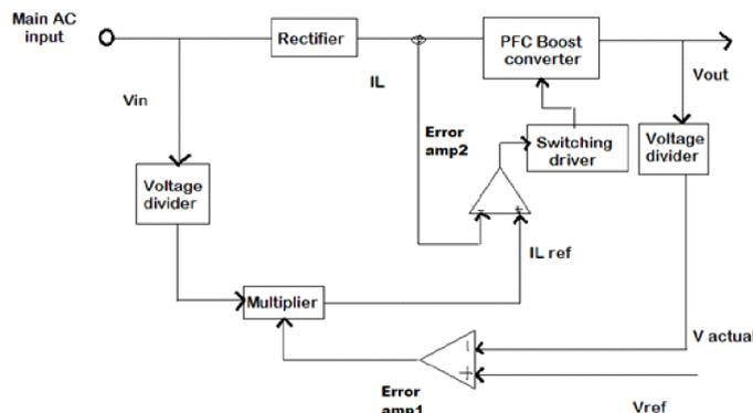
**Figure 4** The PFC control strategy block diagram
