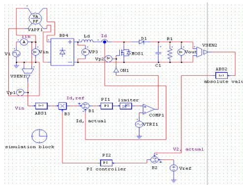
**Figure 11** SMPS using PFC boost converter with  $L_d = 0.005H$
