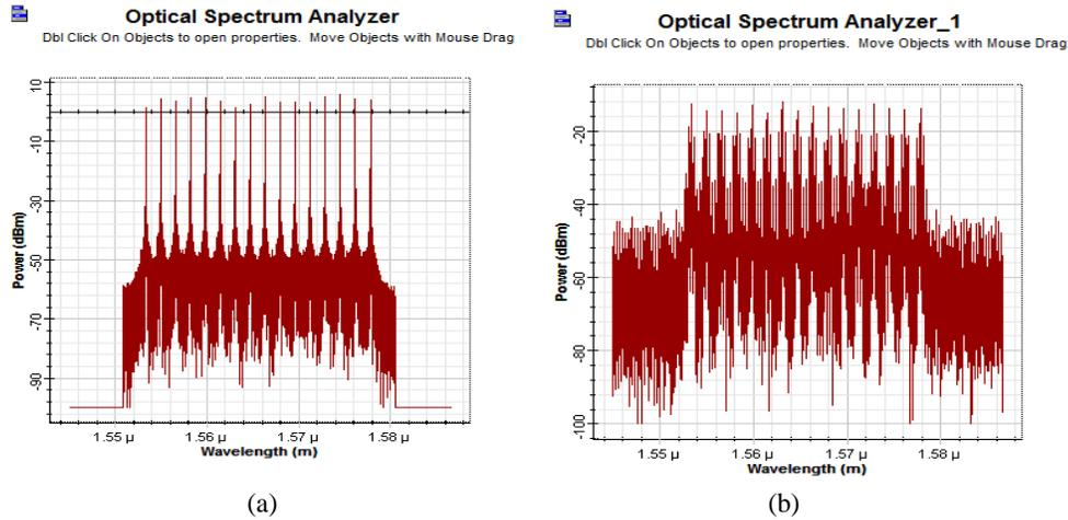
**Figure 8** (a) & (b) shows the Optical spectral analyzer for all 16 channels at Distance 0 km and 1200 km respectively using DRZ Pre compensation technique when Input Power= 5m W & Bit rate= 10 Gbps
