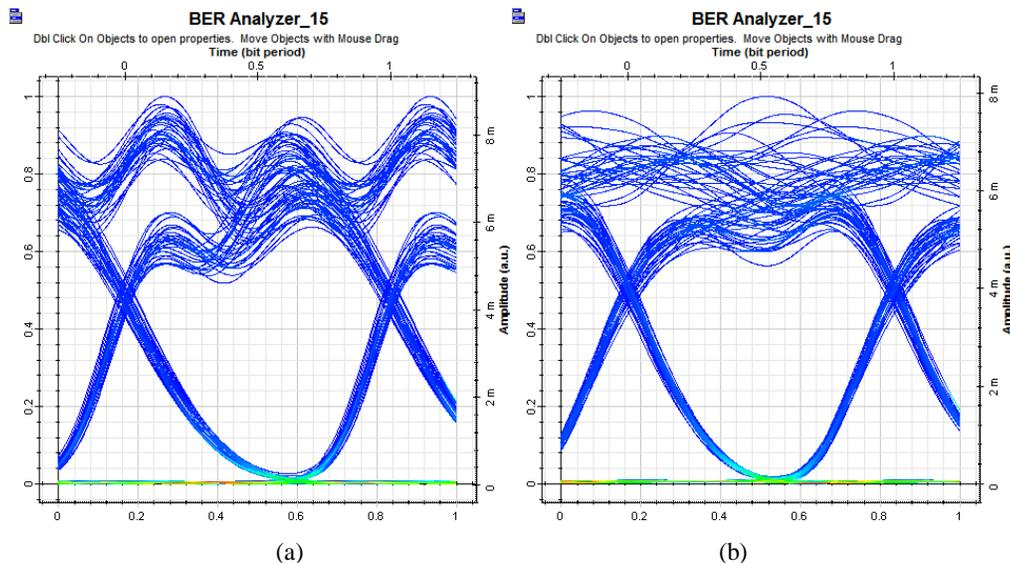
**Figure 3** (a) & (b) shows the Eye diagram of Post compensation CSRZ and DRZ at Power=5m W and Bit rate = 10 Gbps when Distance is 1200 km respectively
