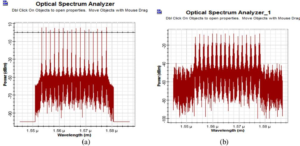
**Figure 7** (a) & (b) shows the Optical spectral analyzer for all 16 channels at Distance 0 km and 1200 km respectively using CSRZ Pre compensation technique when Input Power= 5m W & Bit rate= 10 Gbps
