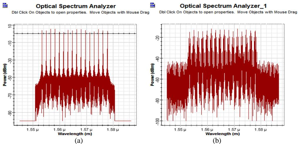
Figure 5 (a) & (b) shows the Optical spectral analyzer for all 16 channels at Distance 0km and 1200 km respectively using DRZ Post compensation technique
