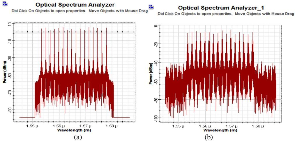
Figure 4 (a) & (b) shows the Optical spectral analyzer for all 16 channels at Distance 0 km and 1200 km respectively using CSRZ Post compensation technique
