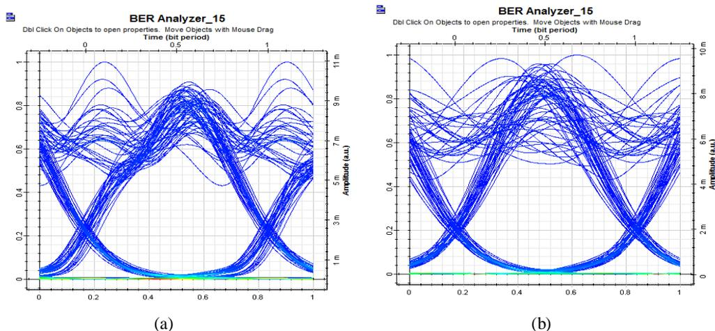
Figure 6 (a) & (b) shows the Eye diagram of Pre compensation CSRZ and DRZ at Power=5m W and Bit rate = 10 Gbps when Distance is 1200 km respectively
